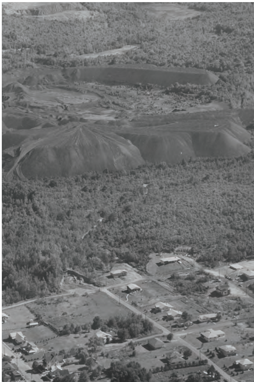
A mountain of culm remaining from mining operations. The location of this culm bank, which was typical of many found throughout the anthracite region, is unknown. Enlargement from a 1970s-era photo. U.S. Bureau of Mines.
