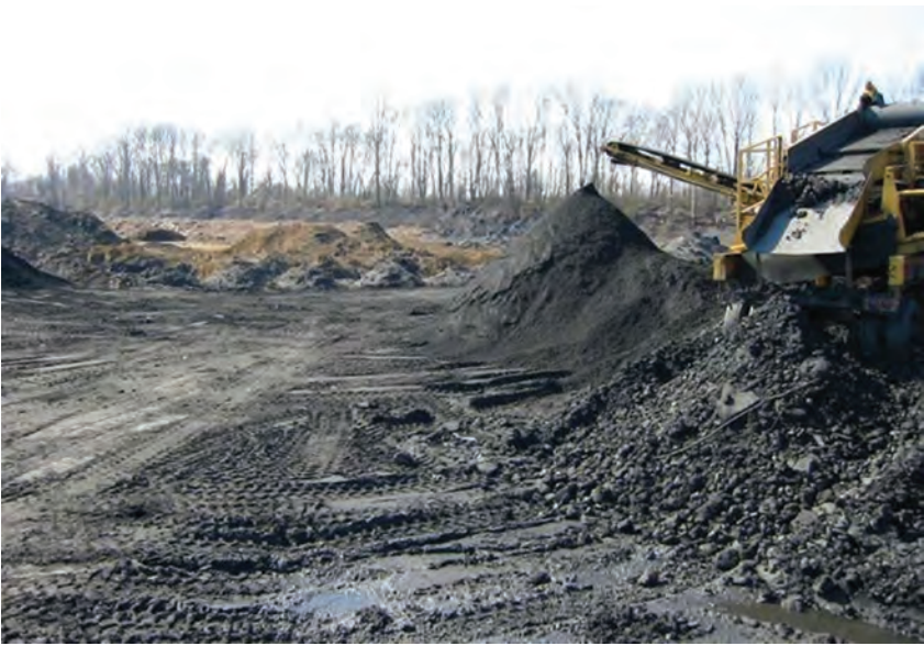
2003 photo showing Stoudt's Ferry Preparation Company reclaiming coal from the Lower Vincent impounding basin. The double deck mobile screen unit, seen at right, separates material into three sizes. Used with permission of the Stoudt's Ferry Preparation Company.
