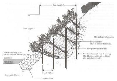
An example of a branch pack design to fill a slumped bank. Source: Engineering Field Handbook
